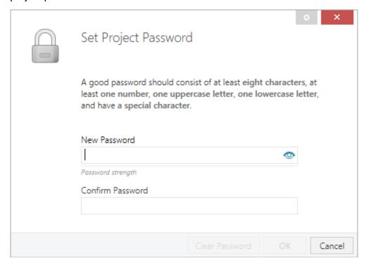
This password protects the ETS project from unauthorized access. This password is not a key that is used for KNX communication. The entry of the password can be bypassed with "Cancel", but this is not recommended for security reasons.
