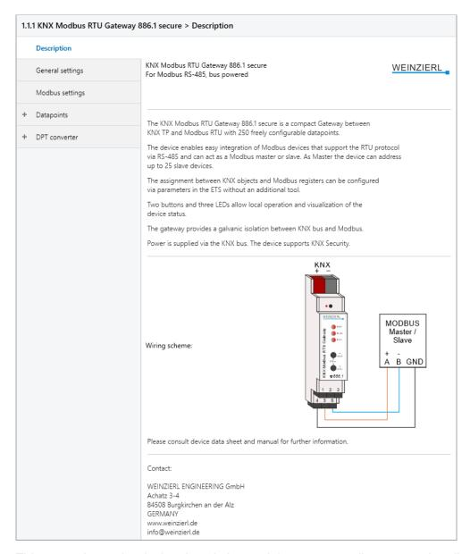
This page shows the device description and the corresponding connection diagram.
