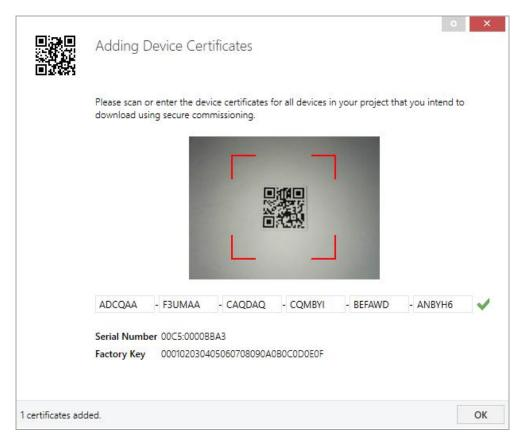
The certificate is printed as text on the device. It can also be scanned from the printed QR code via a webcam.
