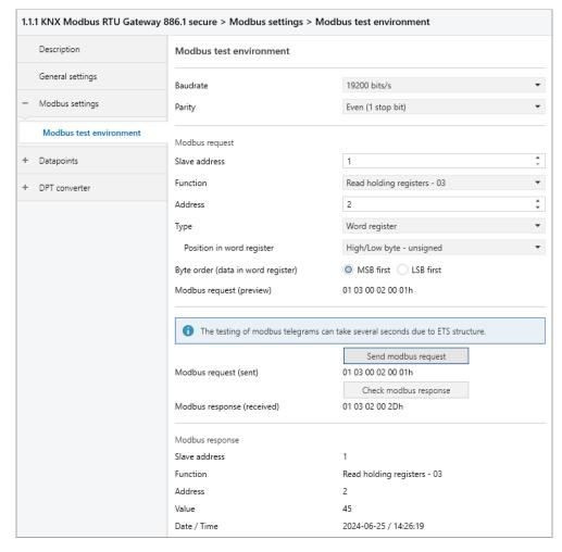
In the Modbus test environment, Modbus telegrams can be created and sent for test purposes. The range of functions corresponds to the settings that can also be used for the individual data points. The names of the parameters are identical.
