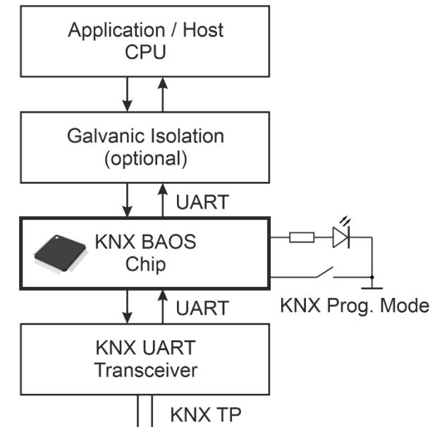
The KNX BAOS Chip does the communication with the KNX bus via a KNX UART transceiver (e.g. Elmos E981.03).
