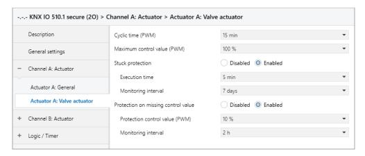
The function valve actuator is foreseen to control thermoelectric valve drives which are used for floor heating but also for radiators. It maps the continuous position (0 % – 100 %) to an ongoing On/Off sequence called PWM (pulse width modulation) signal.
