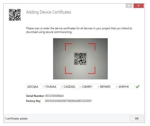
The certificate is printed as text on the device. It can also be scanned from the printed QR code via a webcam.
