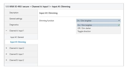
On selection of function Dimming following objects are visible:
