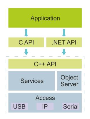
kDrive defines a complete ecosystem for the rapid development of KNX applications on platforms with POSIX (Portable Operating System Interface) operating systems, such as Linux and Windows. Application programming interfaces (APIs) are available in C and .NET.
