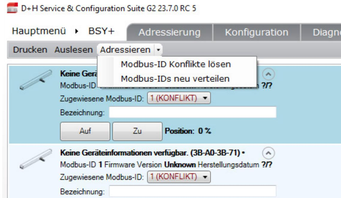
The tool can also be used to easily test the drives and the bus line before they are connected to a Modbus controller or, as in this case, to the KNX Modbus gateway. The use of the tool is described in detail in the document “Modbus addressing of D+H drives with ACB technology”.
