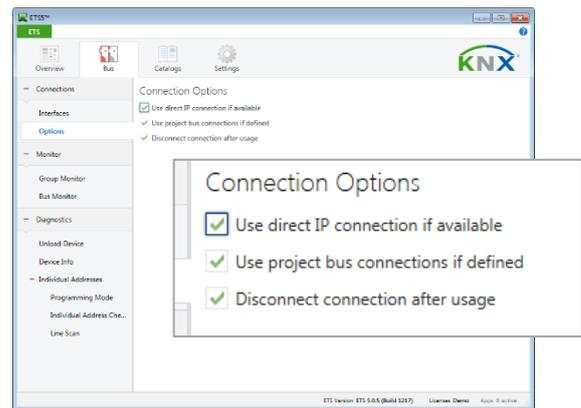
**i** Due to the significantly shorter transmission times it is recommended to perform downloads via IP.
