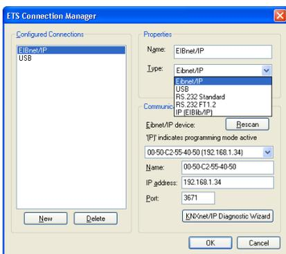
The KNX IP Interface 731 supports up to 5 simultaneous connections. For each connection a separate individual address is used.
