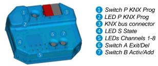
This device is powered only by the KNX bus.
