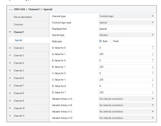
Each channel supports up to 4 valuators to output byte values, or up to 2 valuators to output 2-byte float values:
