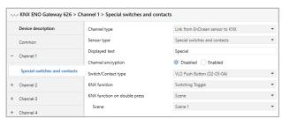
This profile supports push buttons with short/long and double key press. The following object is available for monitoring the battery status:
