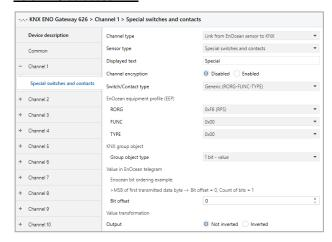
This function can be used to integrate data from EnOcean sensors with EEPs not supported by the gateway, or to evaluate data from sensors with supported EEPs that deviate from the specification.
