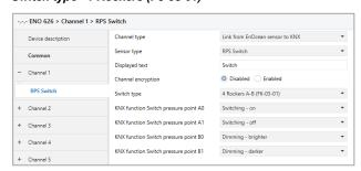
The configuration of a 4-fold rocker is analogous to the 2-fold rocker (F6-02-01), however, it must be noted that for the complete integration, 2 channels must be used in the gateway, one channel for rockers A-B, another channel for rockers C-D. When using a 4-fold rocker, channel encryption is not supported.
