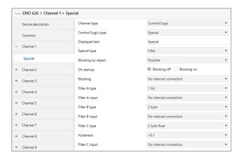
Each channel supports up to 3 filter functions. These functions are primarily intended for internal links to prevent frequent transmission to the KNX bus. The following input types can be selected:
