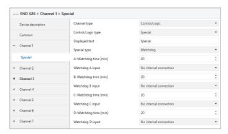
Each channel supports up to 4 functions to monitor the transmission frequency of EnOcean devices:
