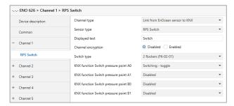
Each pressure point of the 2 rockers can be individually assigned to KNX functions by the parameters "KNX function Switch pressure point":
