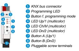
This device is powered by the KNX bus. An external power supply is not necessary.
