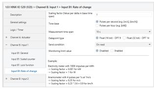
This counter is used to connect devices to the bus where the rate of change is critical within a time interval, e.g. an anemometer.
