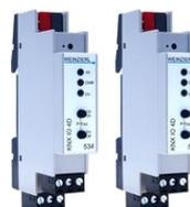
Compact 4-fold dimming actuator with RGB, RGBW and Tunable White (TW) functions. The dimming actuator can be used e.g. for LED panels/strips with RGB / RGBW / Tunable White or for 4 independent dimming channels.
