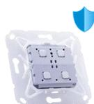
KNX wireless push button of the MATCH 55 series, with integrated bus coupling unit. The wireless push button offers support for EnOcean and KNX RF in one device. The device works in EnOcean mode without configuration (EnOcean Security is activated by a simple push button combination). By configuration with ETS® the push button switches to KNX RF mode and offers optional support of KNX Security.
