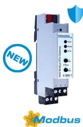
Compact KNX / modbus gateway with 250 freely configurable channels (KNX data points). The device allows easy integration of modbus devices supporting the RTU protocol via RS-485 into KNX installations. It can be used as modbus master or slave. The assignment between KNX objects and modbus registers is done via parameters in the ETS® - no further tool is required. With 2x pluggable screw connectors. One connector can be used with Modbus for the terminating resistor.
